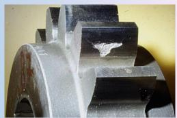
**Test rig:** FZG gear test rig, a = 91.5 mm (ISO 14635)
